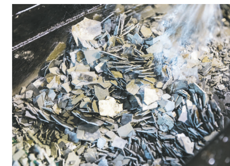
Shards of manganese metal are washed. The shards will then be crushed and eventually shipped to MMC’s customers.
