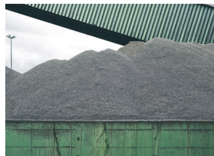
Ore that is used to produce high-purity manganese metal waits to be washed before processing begins at the Manganese Metal Co.
