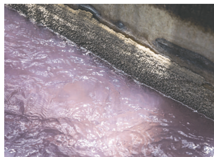
The purple sulfate solution used to dissolve manganese ore at the MMC refinery; the process is used there instead of smelting.
